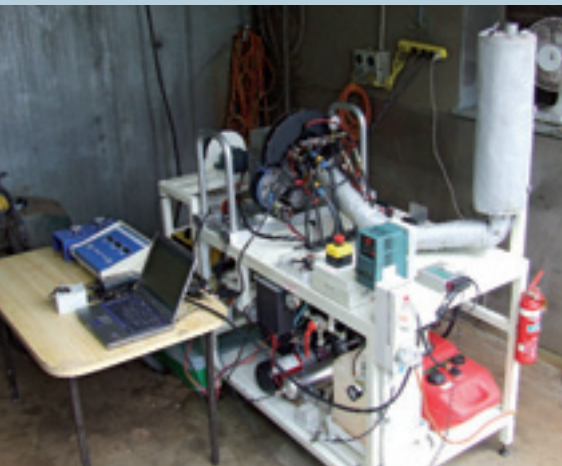
The first 'Stokes' engine working prototype - engineering design, development and testing was undertaken by Queensland-based e3k.
